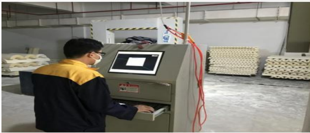
CNC Wire cutting for CG & PIR Pipe section
