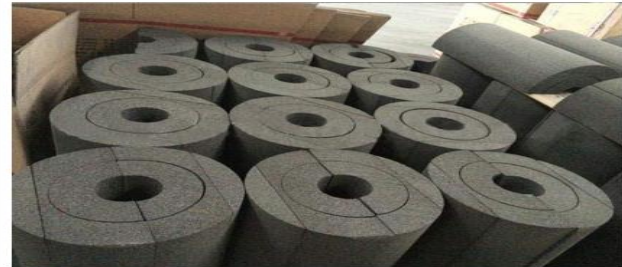
CNC Wire cutting for CG pipe section
