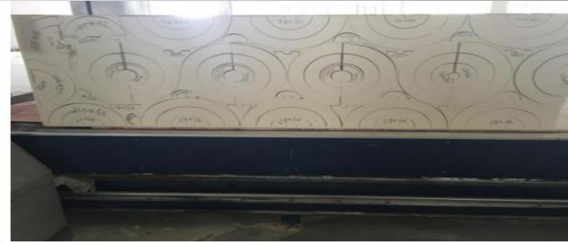
CNC Wire cutting for PIR pipe section
